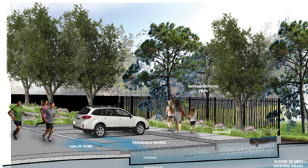
Blue and green infrastructure projects, as shown in these three renderings, use floodwater to manage and enhance greenspaces in urban areas.
